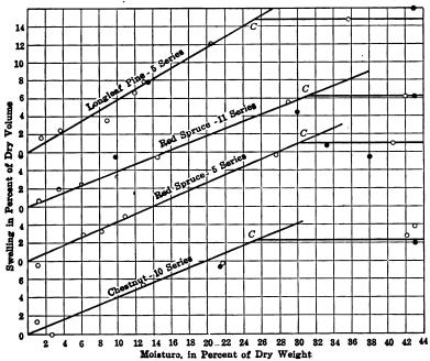
Fig. 60.—Effect of absorption of water on the volume of small, clear pieces of longleaf pine, red spruce, and chestnut. Each point is the average of from 5 to 11 specimens. The fiber-saturation point is at C. The black dots are for specimens that were kiln dried and allowed to reabsorb moisture.
